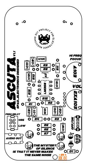
NOW INSERT THE IC IN ITS RESPECTIVE SOCKET PAY ATTENTION TO THE POLARITY EACH IC HAS A HALF MOON OR A SMALL DOT ON PIN 1 PUT IT IN CORRESPONDENCE WITH THE DRAWING ON THE PCB
