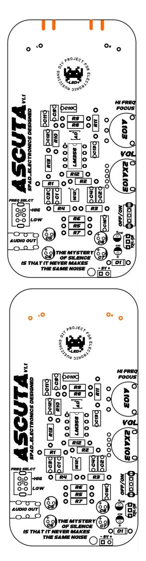
STEP 13 9V BATTERY CLIP: BEFORE SOLDERING THE CABLE, PASS IT THROUGH THE HOLE INDICATED IN THE RED PHOTO AND TIE A KNOT ON ITSELF, THIS WILL PREVENT THE CABLE FROM COMING OFF WHERE IT IS SOLDERED. THEN SOLDER THE RED CABLE ON THE + AND THE BLACK CABLE ON THE -
