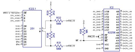
The ROM is wired for the selected 8K block. ROMs larger than 8K can be used with multiple banks being selected by jumpers on the ROM A13,A14 and A15 pins. In most cases, these can be all set high.
