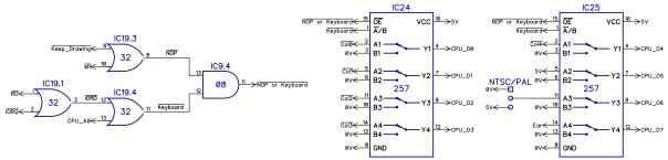
The keyboard is read using bits 0-4 of the input port. There are five column lines, which are pulled high normally. When the keyboard is being scanned, the upper eight address lines are set so that one is low at a time. If a key is pressed on the 5x8 crosspoint keyboard on that row, the column line reads low.
