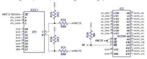
The ROM is wired for the selected 8K block. ROMs larger than 8K can be used with multiple banks being selected by jumpers on the ROM A13,A14 and A15 pins. In most cases, these can be all set high.
