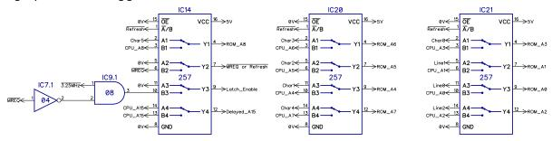
The lower three bits are generated from a line counter, this counts up each line, and is reset on a vertical sync so it is always on line 0 at the start.
