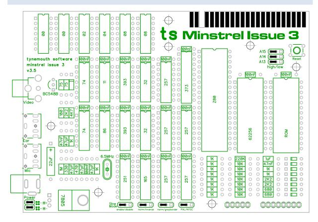
Note on the first run of boards, there are six resistors marked 47K, and one 10K, the design has been revised and 10K should be fitted for all seven of those parts, as shown above.
