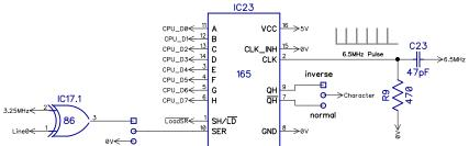
Characters can be inverted by setting bit 7 of the character code. This is latched at the same time as the data is latched into the shift register. During optimisation, this has been implemented using some left over gates, hence the slightly unusual design. A counter is used, if the invert signal is set, there will be a single pulse which will set the output high. Each memory request cycle, the counter will be reset.
