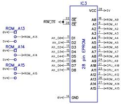
The memory map this creates is as follows, the 8K ROM, mirrored in the upper address space, and 32K RAM with the mirror at the top of RAM used for the display file.
