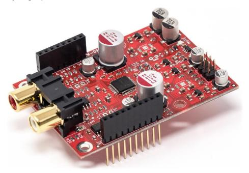
W-DAC 4490 is a very high performance audio DAconverter suitable for high performance DIY DAC setups. Performance figures are very good reaching 119 dBA dynamic range, -108 dB THD+N, and -115 dB THD.
