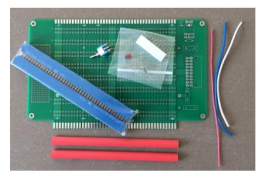
The **Multi-Plane** for EXORbus is a backplane for Motorola EXORbus compatible computer modules, but that's not all! It also includes a fused ATX power connector with switch, can be used as a card extender, and has a small prototyping area (great for developing a small /Page Enable circuit for the Dynamic System Bus of multiple Dynamic RAM Modules).
