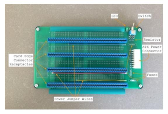
Soldering the large edge connectors on the board can be time consuming and requires a decent quality soldering station for best results. Do not attempt this kit as your first soldering project.
