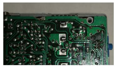
Part of the PCB will need to be filed down slightly to allow clearance for the bolts.
