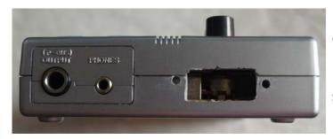
Remove a section of case and drill holes in order to fit the connector in the unit. The exact position may vary based on how the cable has been soldered so it is best to do this at this stage.
