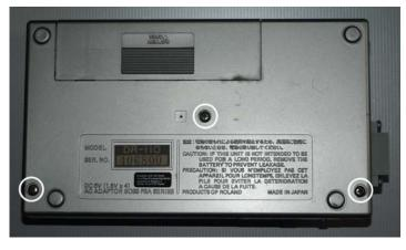
Remove the 3 screws on the base of the DR-110. The back should now come off. Set this aside for later.
