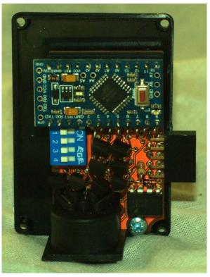
To ensure the PCB has been soldered correctly, the next step is to make and then install the connector for the DR-110 and check the two units work together. This step is very delicate and involves separating and stripping the end of the wires of the ribbon cable so they line up with the pins mentioned in the next section.
