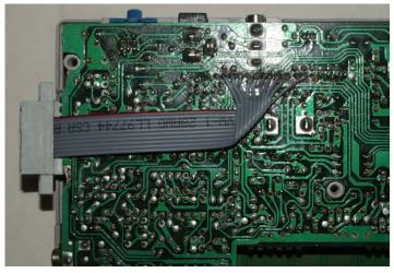
Once soldered, it should look similar to this. At this stage, it is a good idea to connect the mod to the unit to confirm it is working and triggering the sounds properly. If it is not, the soldering must be checked again and possibly redone.
