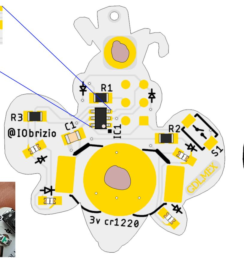
Flip the board Check LED polatity & solder YELIOW LEDS
