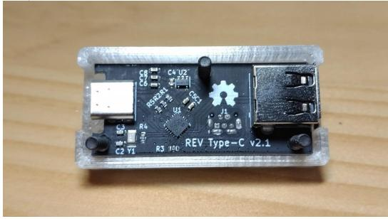
5) Attach the back of the case and screw the M3 nuts onto the bolts. Ensure the board is secured, but make sure the nuts are not overtightened.
