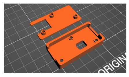
2) Attach adhesive strips to the back of the Adapter case, as shown, and cut the adhesive to provide clearance for the lip
