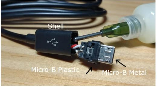
5) Make sure the Micro-B connector is sticking out enough to plug into the robot controller phone. If not, pull on the metal part of the Micro-B connector while also pushing on the plastic part with your fingernail.
