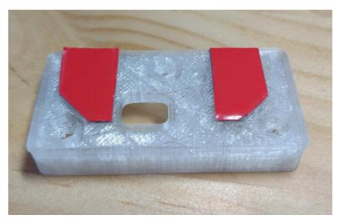
3) Insert M3 hex-head bolts into the case and press the case firmly into a hard surface to seat the bolt heads. If they don't press in nicely, take a pair of tweezers or needle nose pliers and clear out the holes. You may have to push the screws in from the front to clear the hole first.
