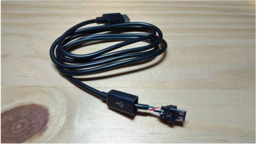
2) (Optional) If you desire charging + OTG functionality on the cable, or would like to enable a special OTG mode through the ID resistor, take the time to desolder the wire bridging the ID pin to ground and carefully solder the resistor of your need on. You must ensure there is adequate spacing inside the shell to fit it.
