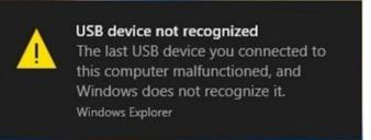
This signifies either a wiring issue between the computer and Adapter, or a faulty Adapter. If you replace the USB cable and this error persists, contact support.
