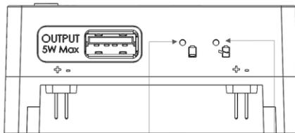
Low battery indicator: amber light turns on when MEGO is in low battery condition.
