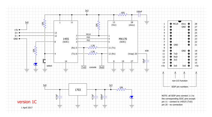
The Explore-28 module contains two LEDs and a **SELECT** button. While one of the LEDs is a power indicator that is permanently lit, the other (mode) LED indicates several different things, depending upon the mode that the 1455 is in.
