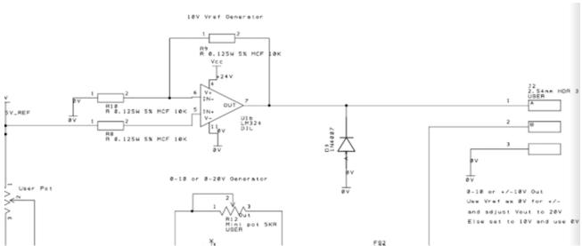
This op amp circuit generates a steady 10V output from the 5V generated by the linear regulator. It's only required when the board is configured to output +/-10V. The output goes to J2-1. The op amp is a non inverting amplifier with a gain of 2.
