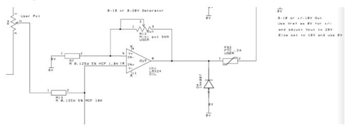
In 0-10V mode R12 is adjusted so that this circuit gives 0-10V output based on the pot position. Requires x2 gain .: R12 = 1K.
