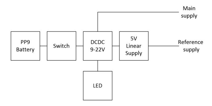
A 9V battery powers a DCDC switching power supply. The DCDC is fed via the side mounted switch (DCDC must go after switch), the output of this is then fed into the main PCB as shown on the schematic. On the main PCB there is a LED which is used to show when the device is turned on and will illuminate off the DCDC output voltage.
