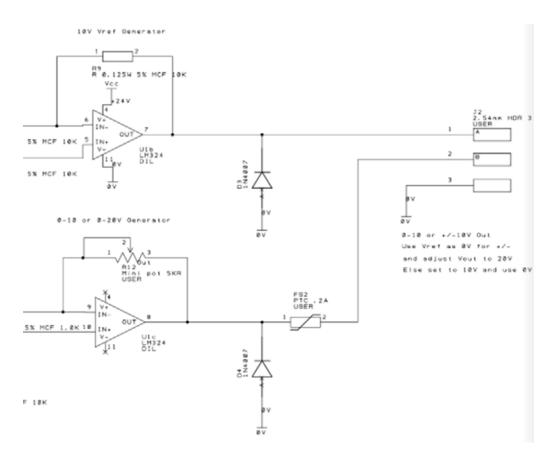
For 0-10V operation J1-3 is taken as the reference voltage and J1-2 is taken as the voltage output to give a 0-10V range.
