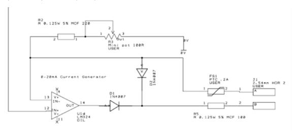
Taking the 20mA case, 5V will be fed into the IN+ terminal from the user pot. IN- must also therefore be at 5V (op amp theory), if this is at 5V then the current through R2+3 must equal 5V/250R = 20mA. Since no current can flow into the IN- terminal then that current must come from the output of the op amp J2-1 into J2-1 via whatever
