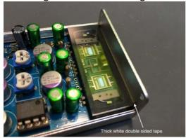
At the edge of Nutube, you will find white thick double sided tape. After finishing solder all parts, please peel thin transparent vinyl tape and fix PCB to metal enclosure. This can avoid too much micro phonic effect of Nutube.
