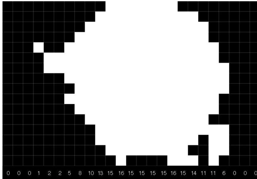
4. **Blob Detection.** Traverse the one-dimensional array of column sums to identify a valid blob. If the column sum is above a defined threshold (`SUM_THRESHOLD`), it will be considered part of the blob. For example, in the image from Step 3, if the threshold is 4, the blob would start at column 7 (which has a sum of 5) and end at column 22 (which has a sum of 6). This is repeated across the entire frame from left to right until all blobs have been detected.
