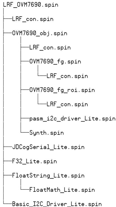
**LRF\_OVM7690.spin** is the top object file. This object handles the user interface, command processing, and laser range finding mathematics.
