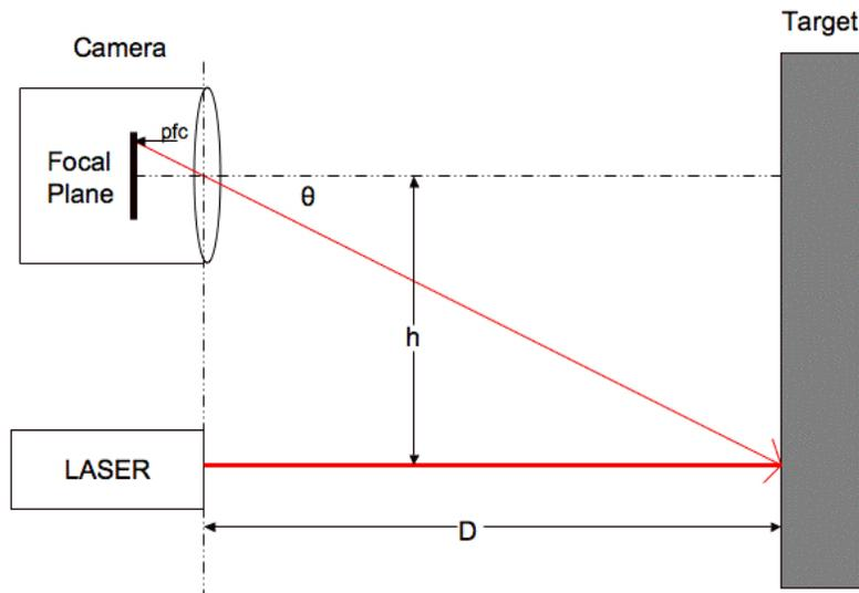
Referring to the figure above, a laser diode module shines a laser spot onto the target object. The value  $h$  is a fixed, known distance between the center points of the laser diode and the camera (78 mm for the LRF Module). When the distance to the target object  $D$  changes, so do both the angle  $\theta$  and the value  $pfc$  (pixels from center), which is the number of pixels the centroid of the primary blob (laser spot) is away from the camera's center point.
