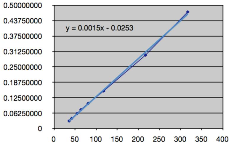
Once the laser is shined onto the target object and the pfc value of the laser spot is received, an angle  $\theta$  can be calculated using the slope-intercept equation and passed to the trigonometric function to determine the actual distance the range finder is from the target object.
