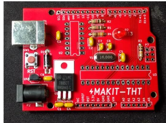
**Step 9:** Bend the leads of the 5V linear regulator as shown:
