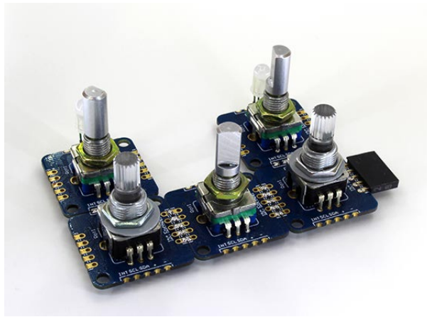
Figure 1.5: Example of 5 boards connected in a matrix with the castellated holes
