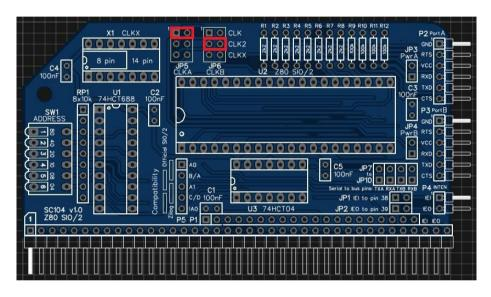
This feature requires software support. This is the standard configuration of clock sources for the RC2014 SIO/2, so most RC2014 software should work.
