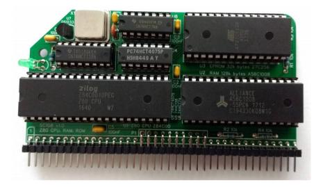
This space saving module is designed to run the Small Computer Monitor, configuration R3, which contains a Machine Code Monitor, BASIC and a CP/M loader.
