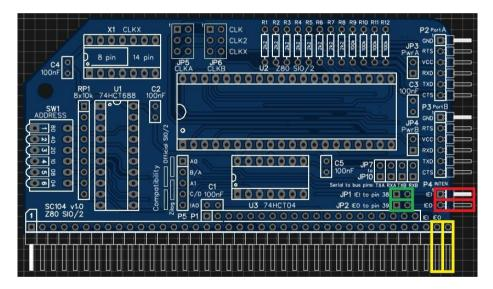
Note that v1.0 of the PCB has the IEI and IEO bus pins incorrectly labelled. It indicates the use of pins 37 and 38, not 38 and 39.
