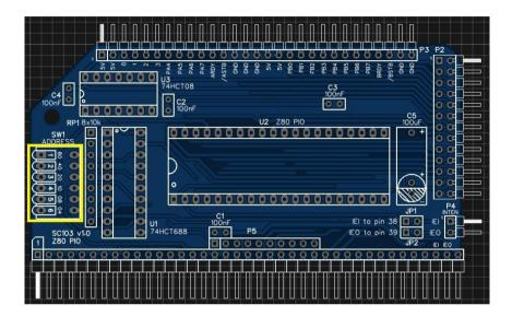
In order to provide some certainty for software it is strongly recommended you set the base address of your first PIO module to 0x68. The module then occupies I/O addresses 0x68 to 0x6B. This is done by setting the switches as illustrated below.
