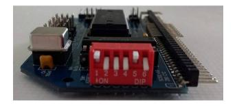
In order to provide some certainty for software it is strongly recommended you set the base address of your first PIO module to 0x68. If you have a second PIO module the recommended base address is 0x6C. If everybody follows this recommendation then software written for the PIO module will know where to find the hardware. The following table shows examples of address switch settings.
