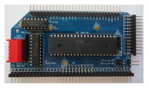
Each port has eight bidirectional data lines and two handshaking lines. The PIO has flexible interrupt generation and fully supports Z80 mode 2 interrupts.
