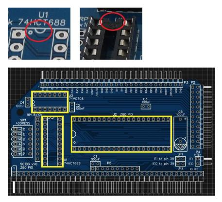
Fit and solder capacitors C1, C2, C3 and C4.
