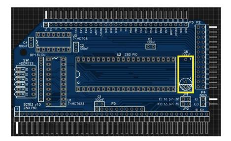
The PCB allows for a radial or axial capacitor. In order to build a low profile board, the capacitor should lay on its side. An axial capacitor would be most secure in this configuration, but there is limited length allocated and you probably don't have one!
