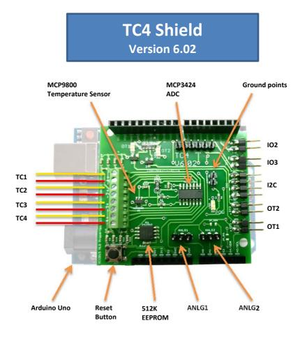
Arduino Uno: The TC4 Shield was intended to be comnnected to an Arduino Uno.
