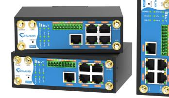
The Ursalink UR75 is an industrial cellular router with embedded intelligent software features that are designed for multifarious M2M/IoT applications. Global WCDMA and 4G LTE carrier supported make this drop-in connectivity a great help for operators in maximizing uptime.
