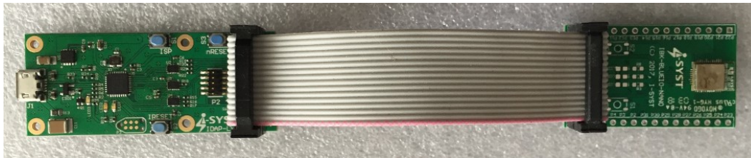
Fig. 6: IDAP-Link JTag with IBK-BLUEIO-NANO for development with the IMM-NRF52832-NANO module
