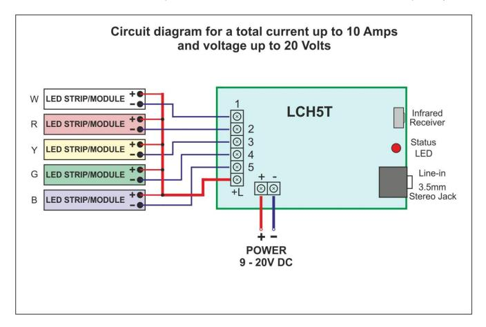
**Note:** First, install spacers in the mounting holes on the board to protect the installed components. **More connection options can be found on the last pages.**
