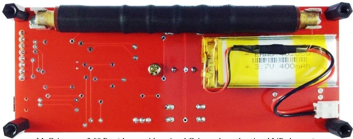
MyGeiger ver. 3.00 Pro (shown with optional Geiger tube and optional LiPo battery)
