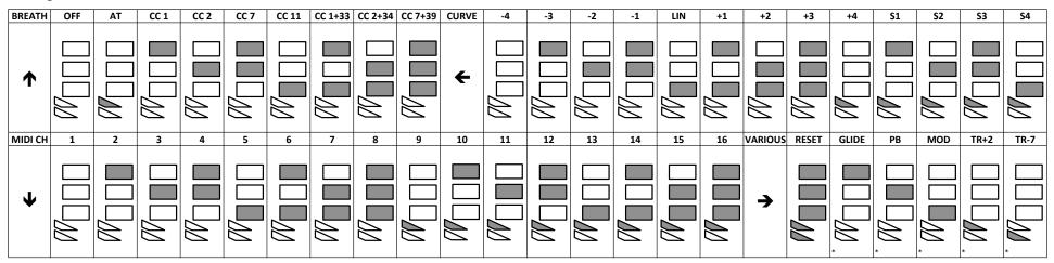
To apply settings: unplug USB, hold joystick in arrow direction, finger the RH combo for the wanted setting and plug in USB. When you see Teensy LED light up, settings have been applied and saved. Release joystick and play. To change another setting, repeat procedure.
