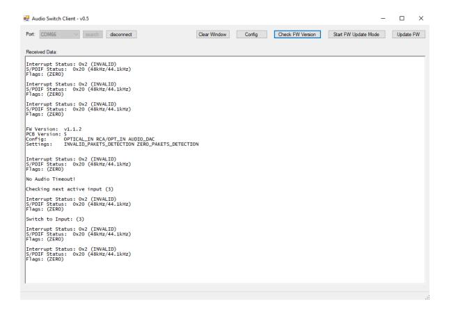
The switch will send status messages every 2 seconds that show the status of the current active input (it is not possible for the audio processor to monitor another input at the same time).
