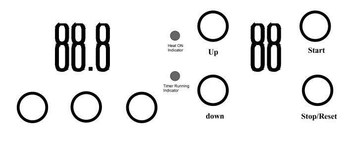
The Thermostat displays the temperature in Celsius, and is pre-set at the factory for 42 degrees Celsius (107 degrees Fahrenheit). It is NOT recommended to use temperature settings above 80 degrees Celsius (176 degrees Fahrenheit).
