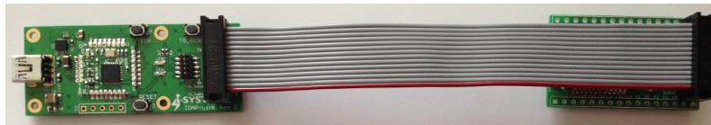
Fig. 2: IDAP-Link™ Rev. 2 connected to the IBK-BLUEIO Rev. 0. Breakout with IMM-NRF51x series module
