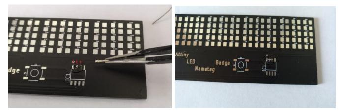
First make a bridge in the first three paths in the top. Use a small piece of wire to help you.
