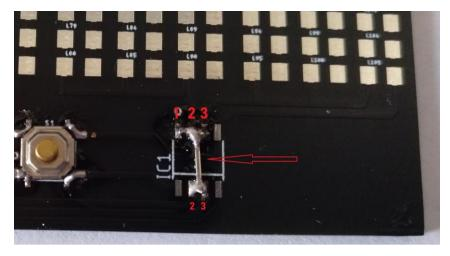
Now bridge the second and third bottom paths, then with a piece of wire join the top and bottom bridges
