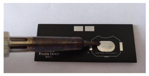
To solder the brooch easier, I recommend you to sand the back down a little bit to make it easier for the solder to stick to it and the path on the board. If you have a powerful soldering iron this might not be needed.
